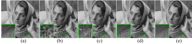
Fig. 17. Image CS results on image Barbara (0.1 N CS measurements). (a) Original image. (b) ReconNet [84] (PSNR = 21.89 dB and SSIM = 0.5732). (c) IST-Net + [86] (PSNR = 23.61 dB and SSIM = 0.6888). (d) CSNet [42] (PSNR = 24.37 dB and SSIM = 0.7217). (e) LGSR (PSNR = 29.40 dB and SSIM = 0.8886).
