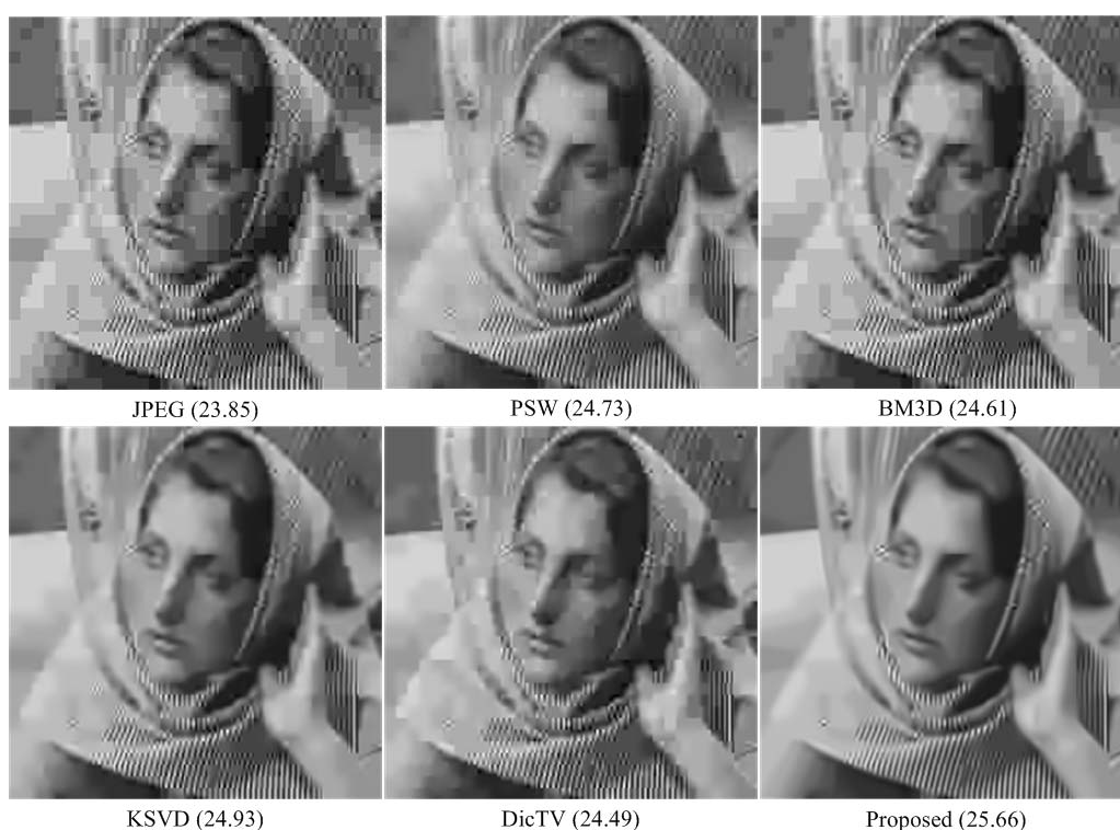
Figure 7. Comparison of tested methods in visual quality on Barbara at QF=5. The corresponding PSNR values (in dB) are also shown.
