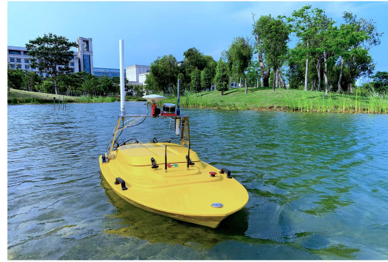
Fig. 14. Surface vessel Q-Boat 1800P used for operations on a lake at the University of Macau.
