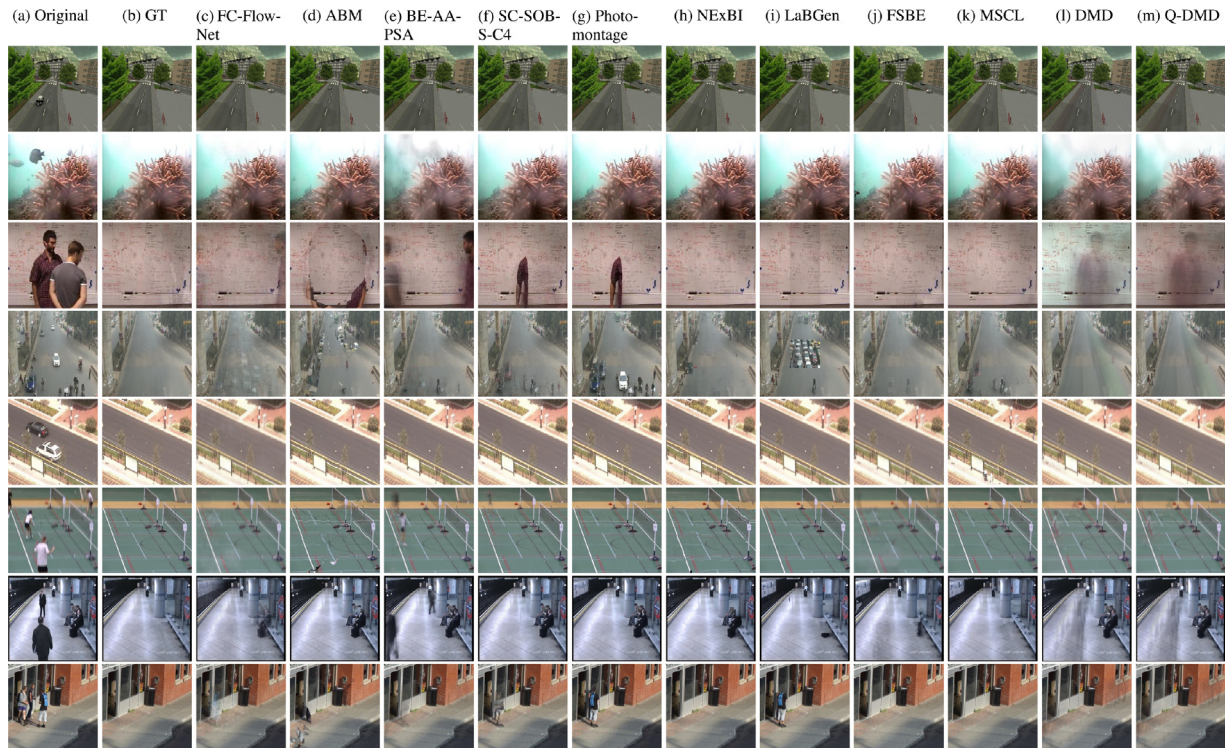
Fig. 2. (a) Representative original frames of the eight videos from the SBMnet dataset. (b) Ground truth of the background. (c)–(m) are the generated backgrounds results of FC-FlowNet, ABM, BE-AA-PSA, SC-SOBS-C4, Photomontage, NExBI, LaBGen, FSBE, MSCL, DMD, Q-DMD, respectively. From top to bottom: First-row: 511; Second-row: Blurred; Third-row: board; Fourth-row: boulevardJam; Fifth-row: boulevard; Sixth-row: Badminton; Seventh-row: AVSS-2007; Last-row: BusStation.
