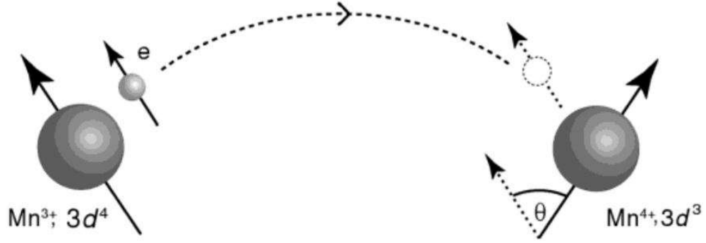
Figure 2.10: The double exchange interaction. The electron hops with spin memory from one localized ion core to the next [158].
